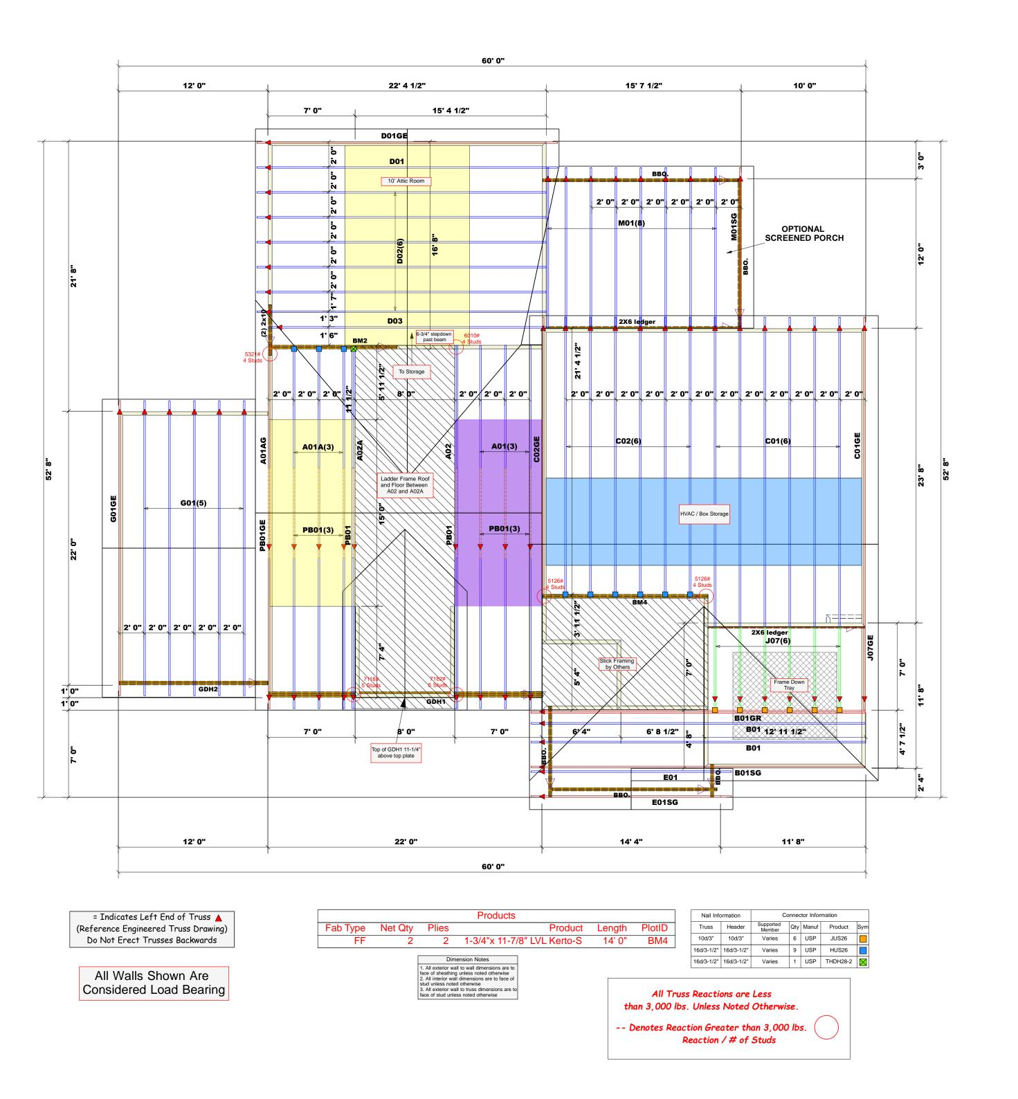
ROOF & FLOOR TRUSSES & BEAMS
