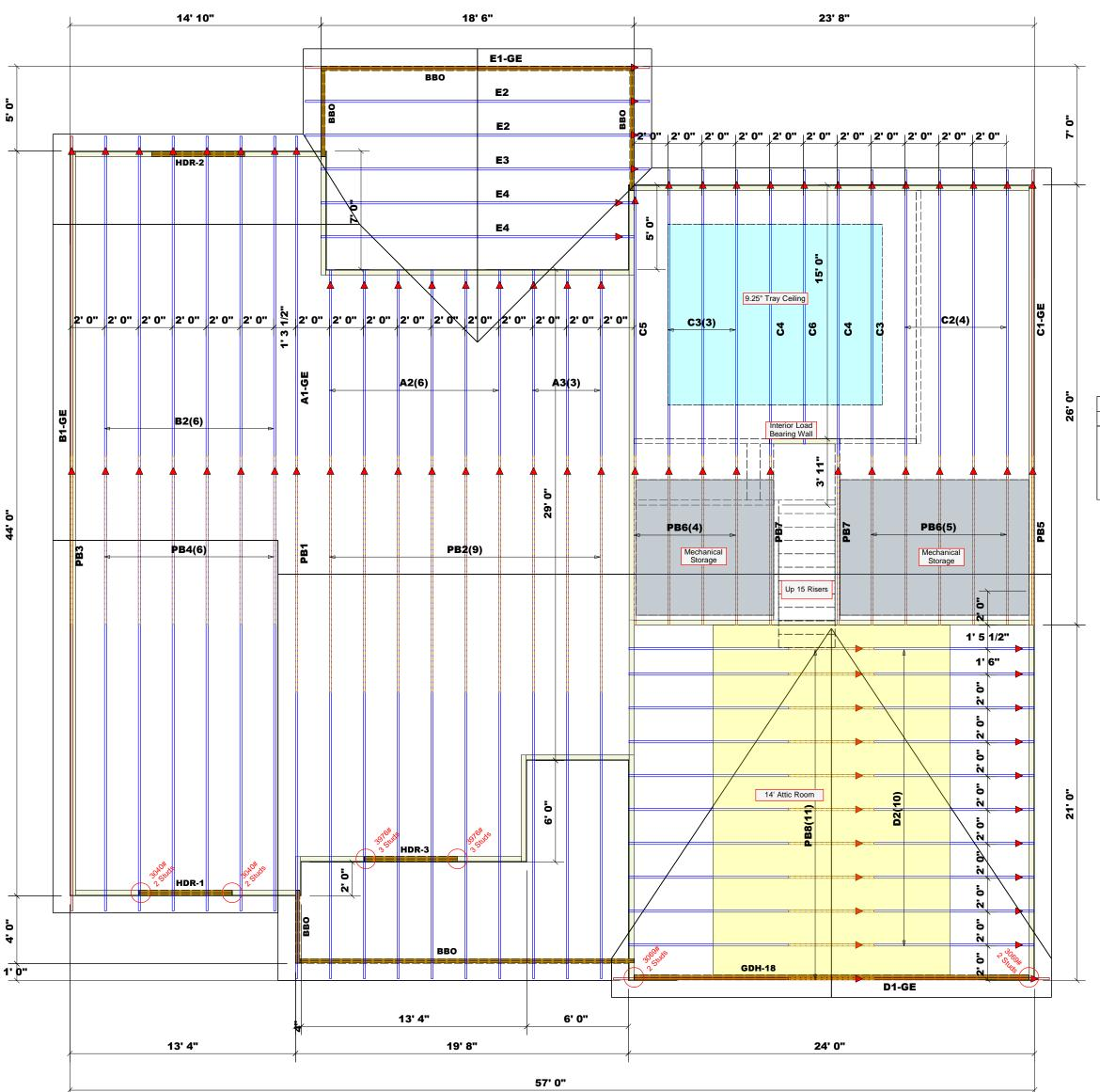
▲ = Indicates Left End of Truss (Reference Engineered Truss Drawing) Do Not Erect Trusses Backwards
