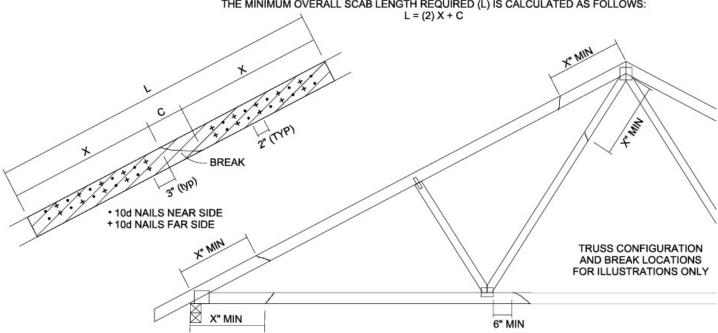
THE LOCATION OF THE BREAK MUST BE GREATER THAN OR EQUAL TO THE REQUIRED X DIMENSION FROM ANY PERIMETER BREAK OR HEEL JOINT AND A MINIMUM OF 6" FROM ANY INTERIOR JOINT (SEE SKETCH ABOVE)
