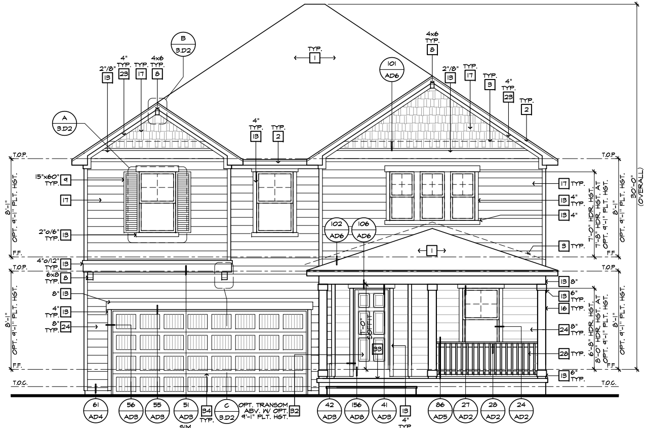
FRONT ELEVATION 'D' W/ CRAWL SPACE SCALE 1/4"=1'-0" (22"x34") - 1/8"=1'-0" (11"x17")
