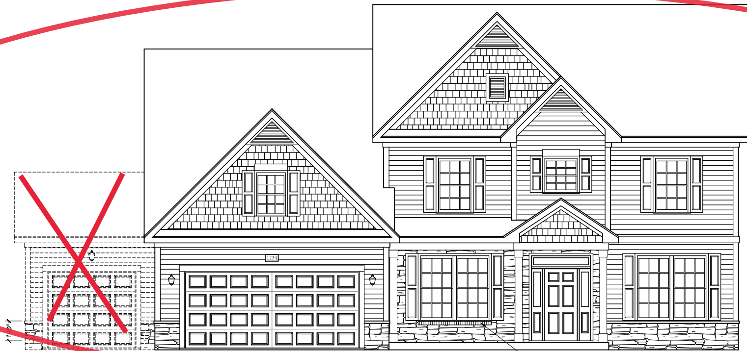
FRONT ELEVATION-A-3 SCALE: 1/4" = 1'-0" BRICK OR STONE LEDGE AS SPEC. (TYP.)
