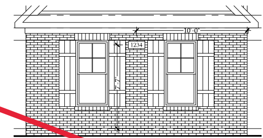
Front Elevation W/ Opt 2-Car & Opt 1-Car side load Garage SCALE: 1/4"=1'-0" ON 22x34 AND 1/8"=1'-0" ON 11x17
