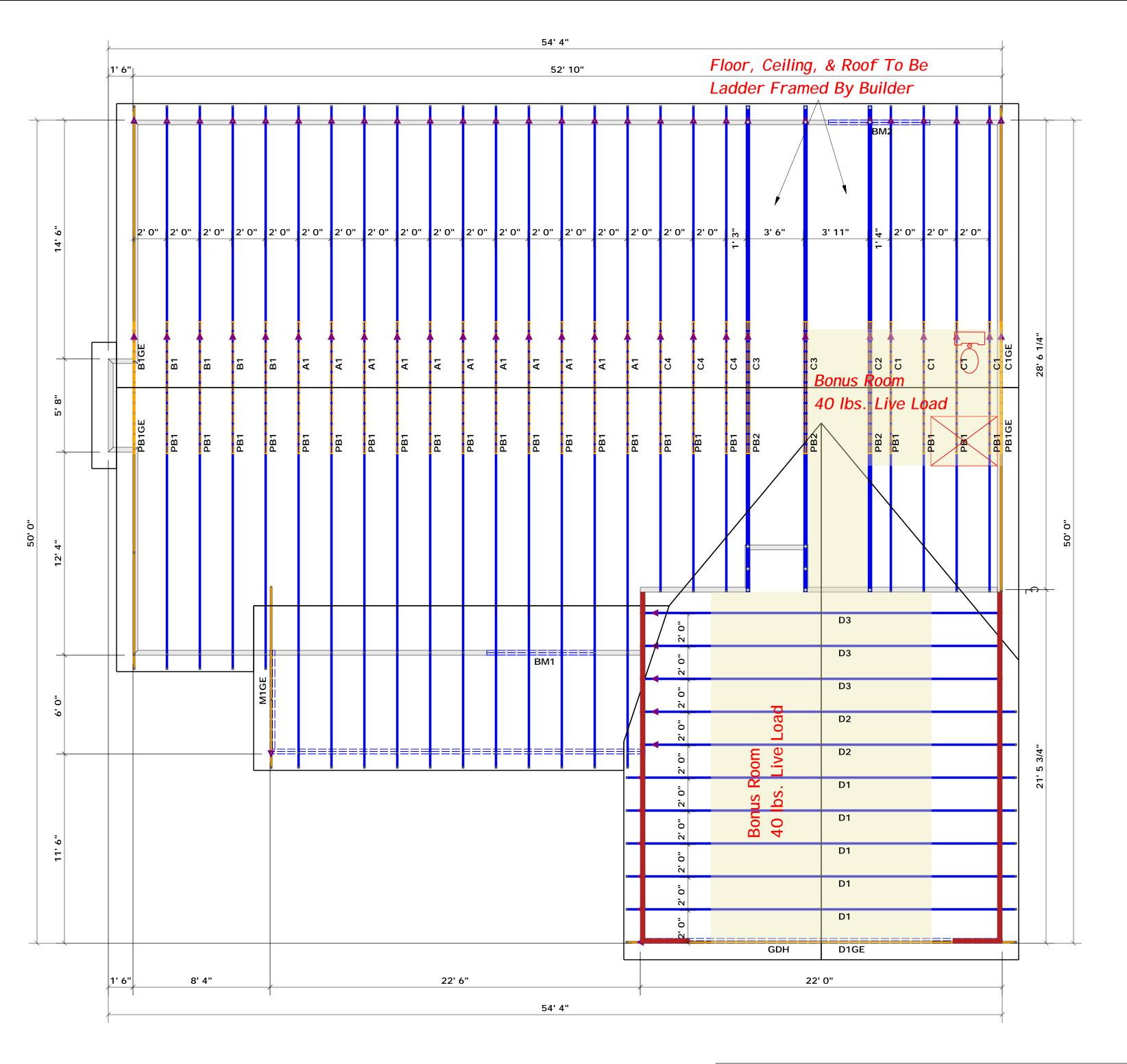
▲ = Denotes Left End of Truss(Reference Engineered Truss Drawing)Do Not Erect Trusses Backwards
