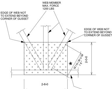
\* MEASUREMENT TAKEN AT POINTS WHERE WEB ACHIEVES FULL MEMBER DEPTH (AS MEASURED PERPENDICULAR TO WEB'S SAW-MILLED EDGE)
