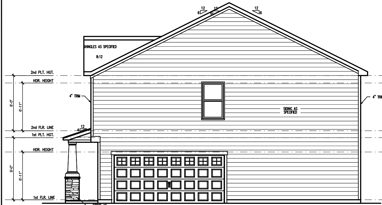
OPT. 2-CAR SIDELOAD GARAGE RIGHT SIDE ELEVATION 'CRAFTSMAN' (SLAB) SCALE: 1/4" = 1'-0" ON 22x34, 1/8" = 1'-0" ON 11x17
