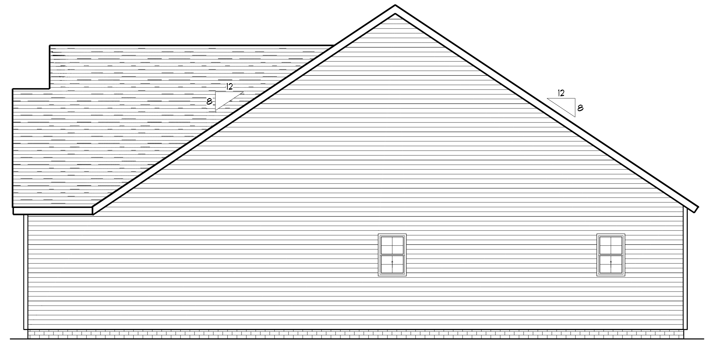
RIGHT ELEVATION SCALE: 1" = 1/4"
