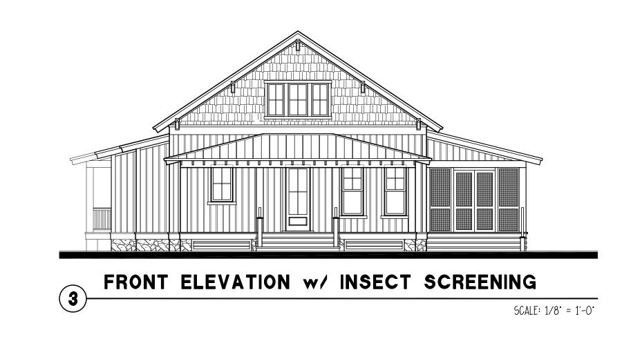
5v MTL. ROOFING. typ. — EXPOSED P.T. — RAFTER TAILS RIDGE w/ VENT — \_\_\_\_\_\_ J BASE PLATE HT. FIELDSTONE VENEER OVER P.T. HORIZONTAL P.T. WD. STEPS. typ. CMU BLOCK PIER. FRONT ONLY HOGSPEN SCREENING SERVICE YARD, SEE DETAIL 6, SHEET 6 - — ADJUST HEIGHT TO SCREEN ALL UTILITIES P.T. WD. BAND P.T. 6° CORNER + DRIP BOARD BOARD, typ. PARGE COAT OVER P.T. WD. RAILS
