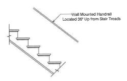
Stair Detail 16 Risers @ 7-3/4" W/ 15 Treads @ 10" + 1" Nosing
