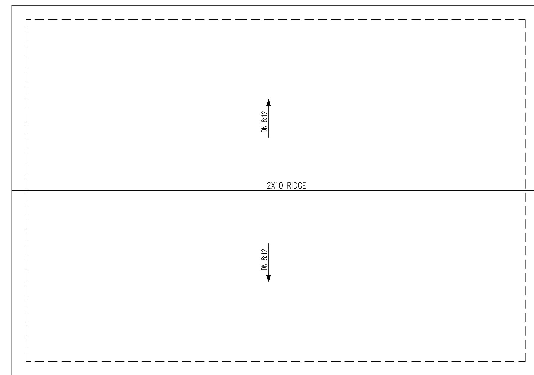
ROOF FRAMING PLAN 1/4" = 1'-0"
