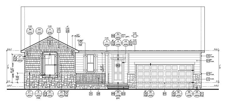
FRONT ELEVATION 'B' W/ STONE AT CRAWL SPACE AT OPTIONAL 9'-I" PLT. HGT.
