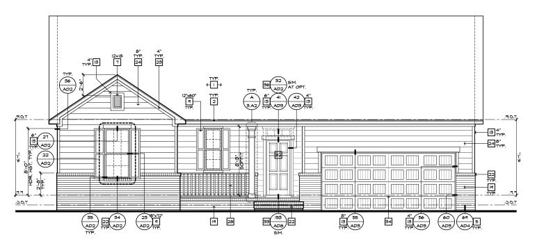
FRONT ELEVATION 'A' W/ BRICK AT CRAWL SPACE AT OPTIONAL 9'-I" PLT. HGT.
