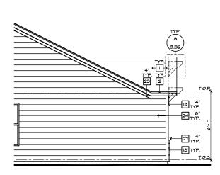
PARTIAL LEFT ELEVATION 'B' W/ STONE OPTION SCALE I/4"=1'-0" (22"X34") - I/8"=1'-0" (II"XI7")
