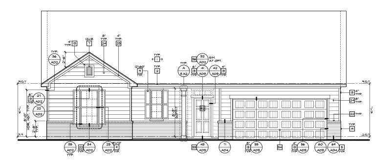
FRONT ELEVATION 'A' W/ BRICK AT OPTIONAL 9'-I" PLT. HGT.
