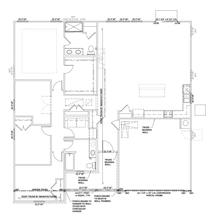
INTERIOR LOAD BEARING WALL - ROOF RAFTER / TRUSS SUPPORT ----- DOUBLE RAFTER / DOUBLE JOIST
