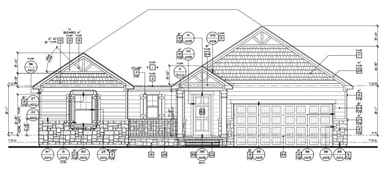
FRONT ELEVATION 'C' W/ STONE AT CRAWL SPACE
