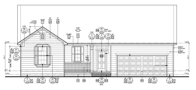
FRONT ELEVATION 'A' W/ CRAWL SPACE AT OPTIONAL 9'-I" PLT. HGT.
