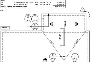
PARTIAL ROOF PLAN SCALE 1/8"=1'-0" (22"X34") - 1/16"=1'-0" (11"X17")
