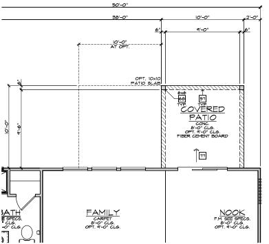
PARTIAL ROOF PLAN PARTIAL SLAB INTERFACE PLAN SCALE 1/8"=1'-0" (22"X34") - 1/16"=1'-0" (11"X17") SCALE |/4"=|'-0" (22"X34") - |/8"=|'-0" (||"X|7")
