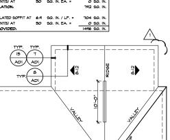
PARTIAL ROOF PLAN SCALE 1/8"=1'-0" (22"X34") - 1/16"=1'-0" (11"X17")
