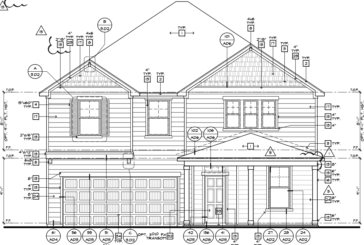
FRONT ELEVATION 'D' AT OPTIONAL 9'-1" PLT. HGT.
