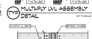
TYP ASSEMBLY BOLTING AT MULTI-PLY LVL BEAM TO BEAM CONNECTIONS
