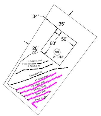
System: Gravity to Serial Dist. Lines: 4—8, (355') Accepted Status System 0.35 Soil LTAR
