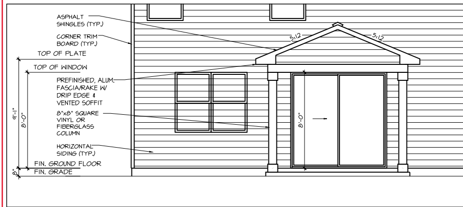
COVERED PORCH PPO - REAR ELEVATION
