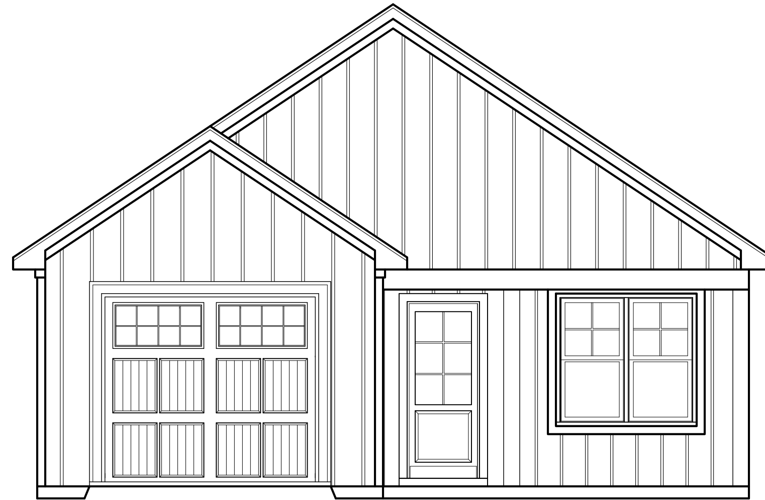
FRONT ELEVATION 1/4" = 1'-0" *MONO SLAB*
