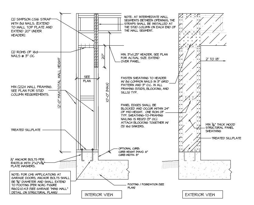
905B CS-PF: CONTINUOUS PORTAL FRAME CONSTRUCTION
