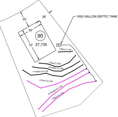
System: Gravity to Serial Dist. Lines: 5-7, (400') Accepted Status System 18" Trench Bottom 0.35 Soil LTAR
