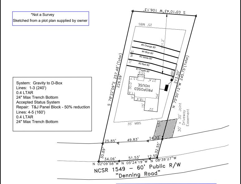
\*\*1000 Gallon Septic Tank Tank and trenches to be located minimum of 10' from any property line and minimum of 5'
