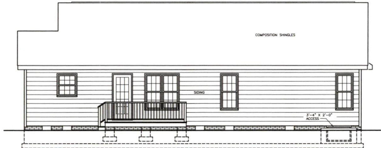
REAR ELEVATION SCALE : 1/4"=1'-0"
