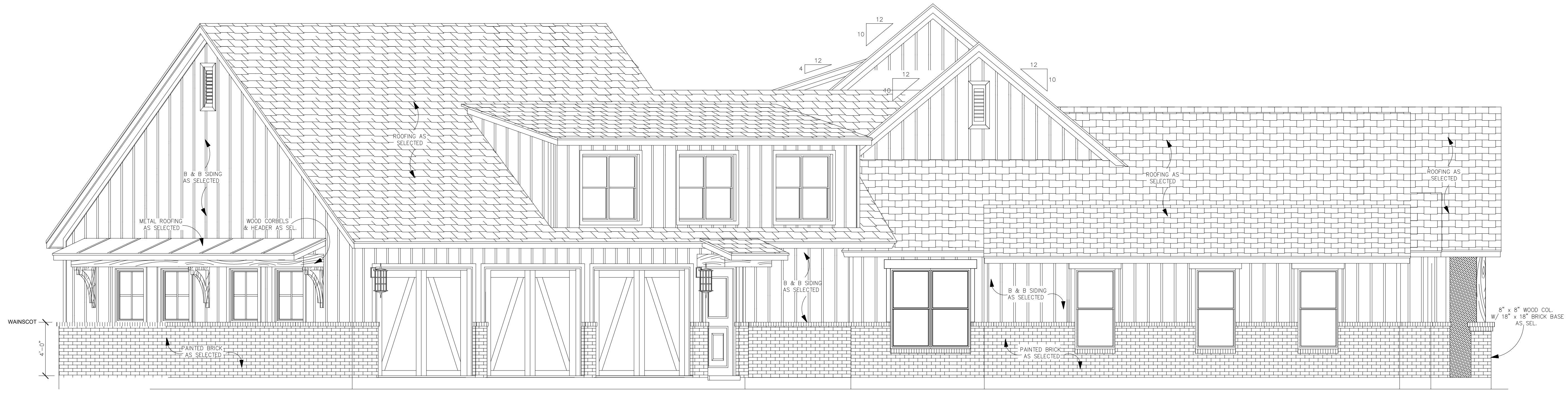
RIGHT ELEVATION SCALE 1/4" = 1'-0" NOTES: - PROVIDE MEP - DRAWINGS INDICATE A IF FLOOR SYSTEM
