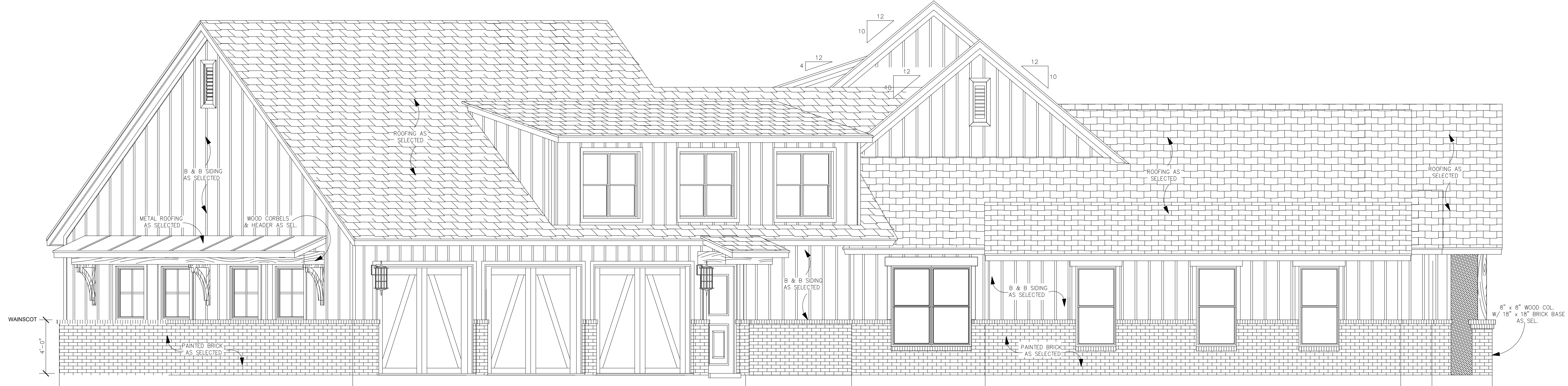
RIGHT ELEVATION SCALE: 1/4" = 1'-0" NOTES: - PROVIDE MEP HULLS #4F 02 - DRAWINGS INDICATE A 1" FLOOR SYSTEM
