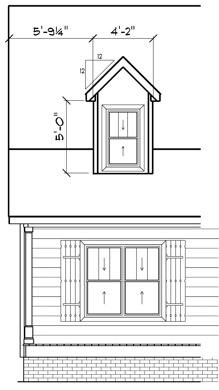
DORMER DETAIL PLAN SCALE: 1" = 1/4"
