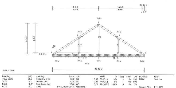
7) This truss is designed in accordance with the 2015
