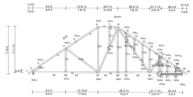
Plate Offsets (X, Y): [2:0-3-5,0-0-3], [6:0-4-4,0-2-4], [8:0-7-12,0-2-0], [10:0-3-0,0-3-0], [17:0-11-11,0-2-8], [18:0-3-5,0-0-3], [18:1-9-11,0-2-0], [26:0-3-0,0-3-0], [27:0-3-12,0-3-0] (psf) Spacing 2-0-0 CSI DEFL Loading (loc) I/defl L/d PLATES GRIP
