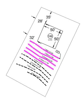
System: Gravity to D-Box Lines: 1-3, (3x90'x3') Accepted Status System 0.35 Soil LTAR
