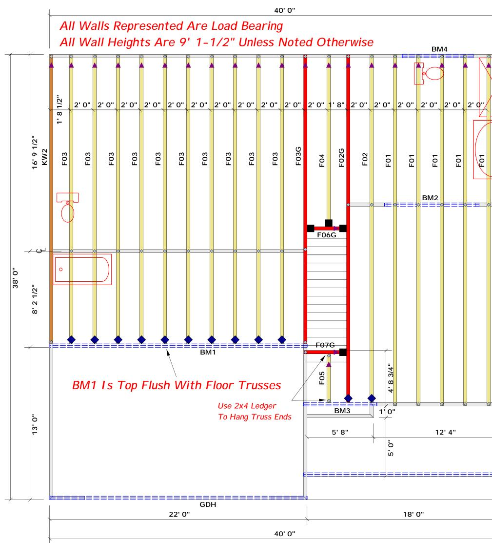
= Denotes Left End of Truss (Reference Engineered Truss Drawing) Do Not Erect Trusses Backwards
