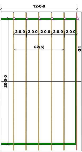
Truss Placement Plan SCALE: NTS = Indicates Left End of Truss(Reference Engineered Truss Drawing)Do NOT Erect Truss Backwards
