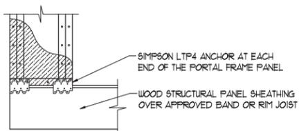
OVER RAISED WOOD FLOOR - FRAMING ANCHOR OPTION
