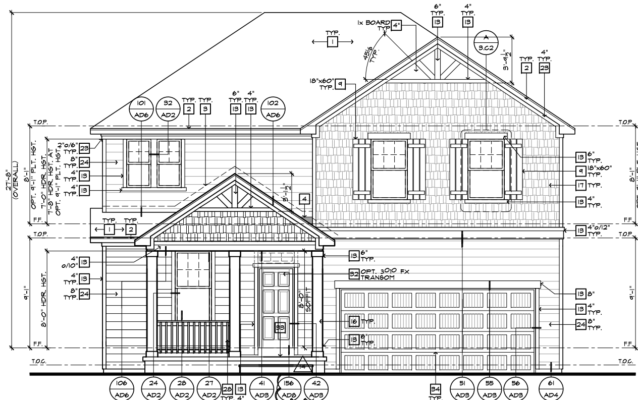
FRONT ELEVATION 'C' W/ CRAWL SPACE AT OPTIONAL 9'-1" PLT. HGT. SCALE 1/4"=1'-0" (22"X34") - 1/8"=1'-0" (11"X17")
