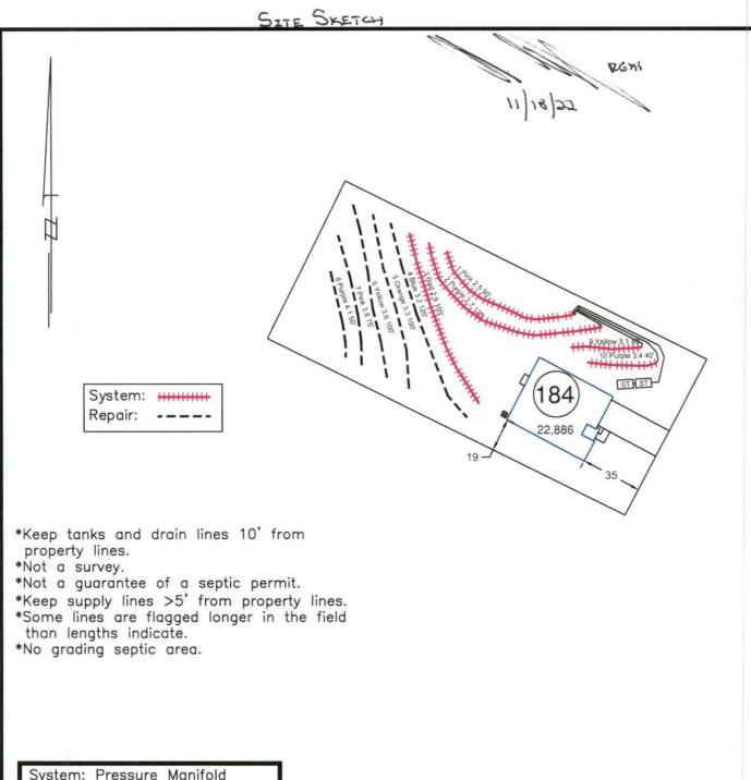
System: Pressure Manifold Lines: 3-6, (400') Accepted Status System 0.3 Soil LTAR
