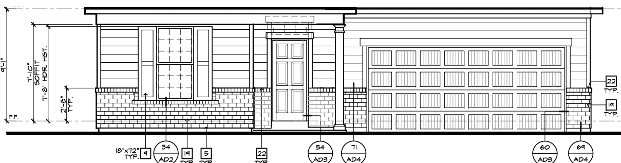
PARTIAL FRONT ELEVATION 'A' AT OPTIONAL 9'-1" PLT. HGT. W/ STONE OPT. SCALE 1/4"=1'-0" (22"X34") - 1/8"=1'-0" (11"X17")
