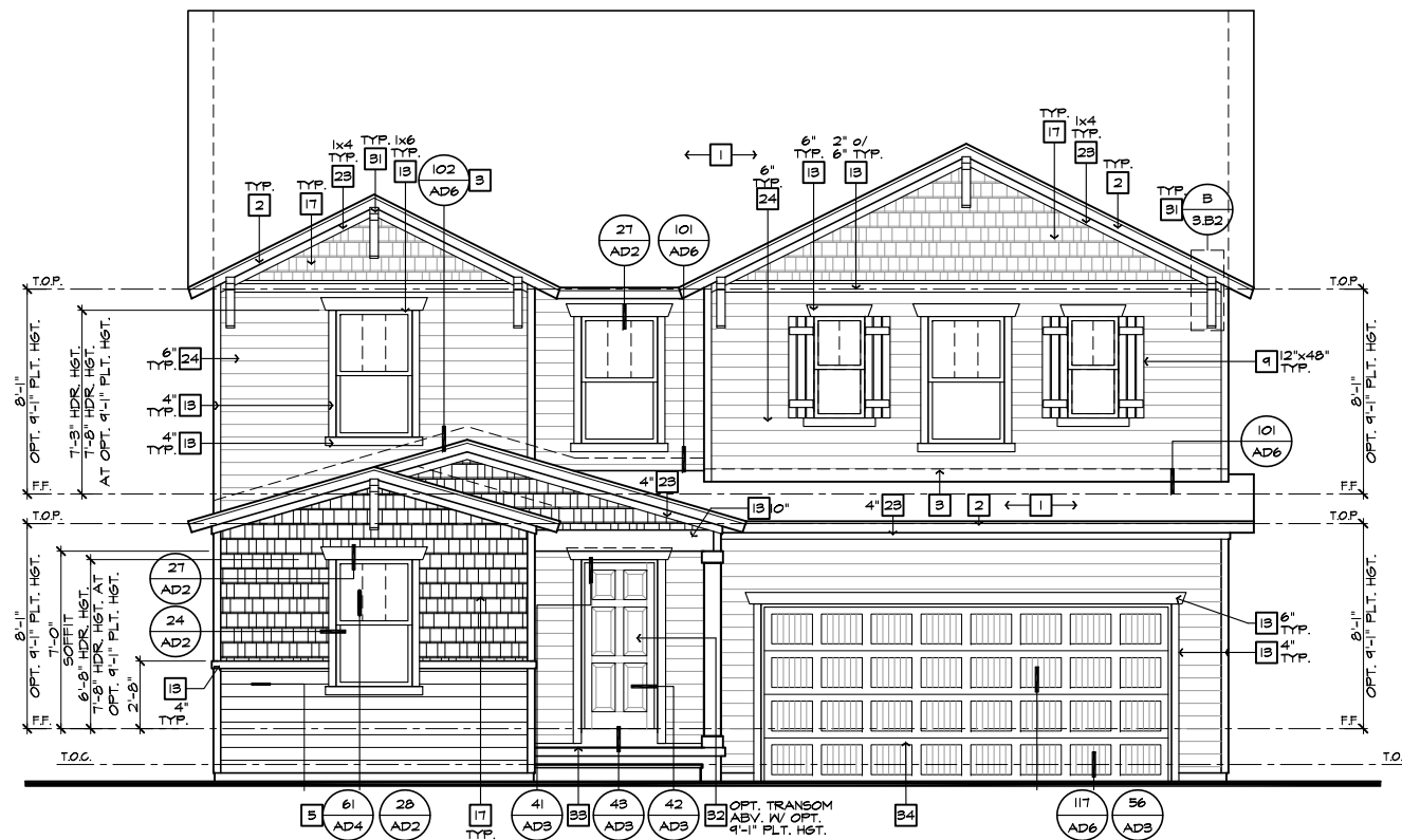
FRONT ELEVATION 'B' W/ CRAWL SPACE
