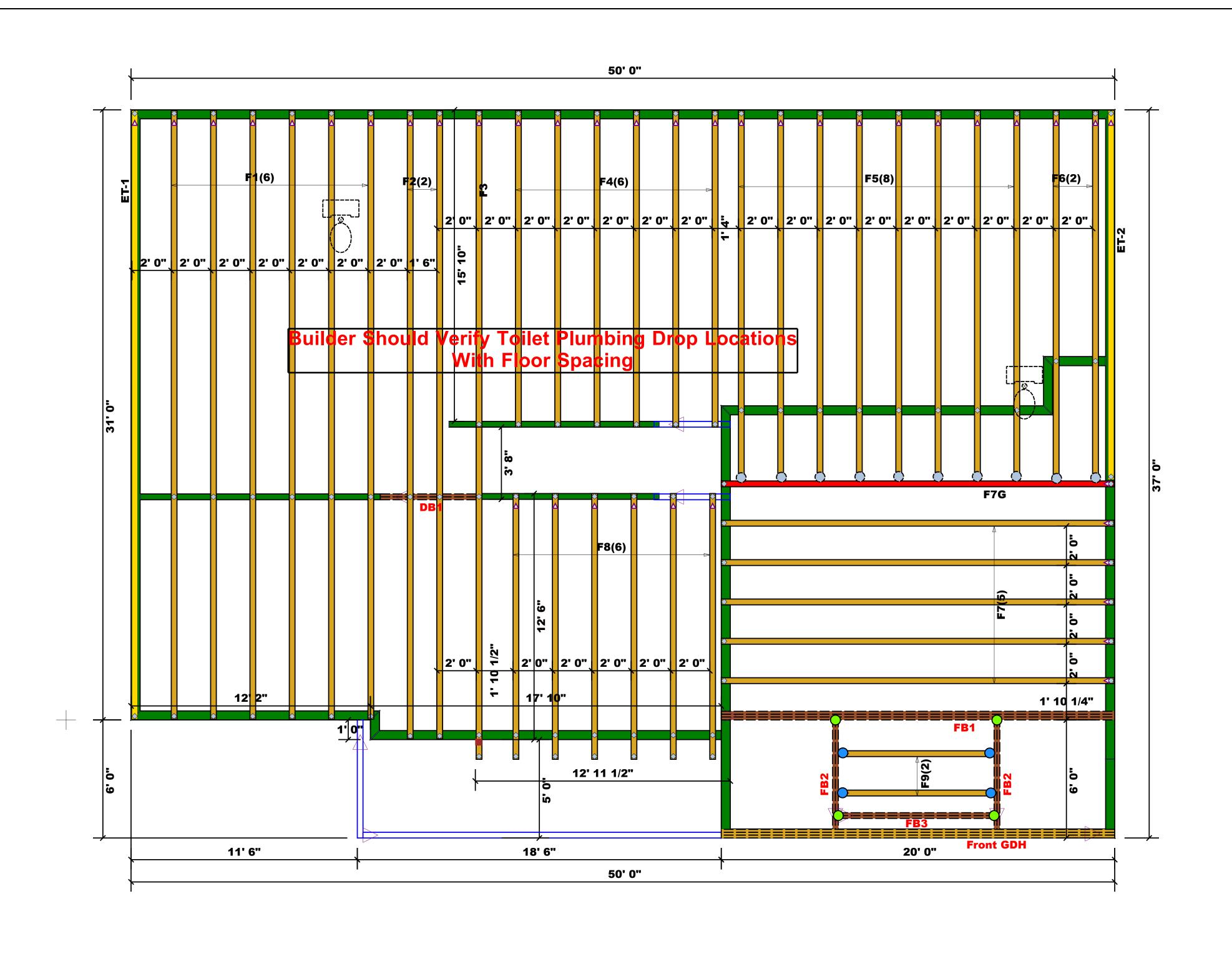
= Indicates Left End of Truss (Reference Engineered Truss Drawing) Do NOT Erect Truss Backwards
