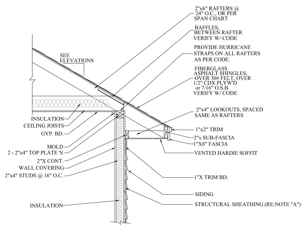
NOTE "A": PROVIDE A MINIMUM OF 7/16" STRUCTURAL WOOD PANEL ATTACHED w/ 8d COMMON OR 10d BOX NAILS AT 4" SPACING ON EDGE AND 12" IN FIELD. NOTE "B": CORNICE DETAIL FOR REFERENCE ONLY. REFER TO BUILDER SPECS FOR ACTUAL MATERIALS.
