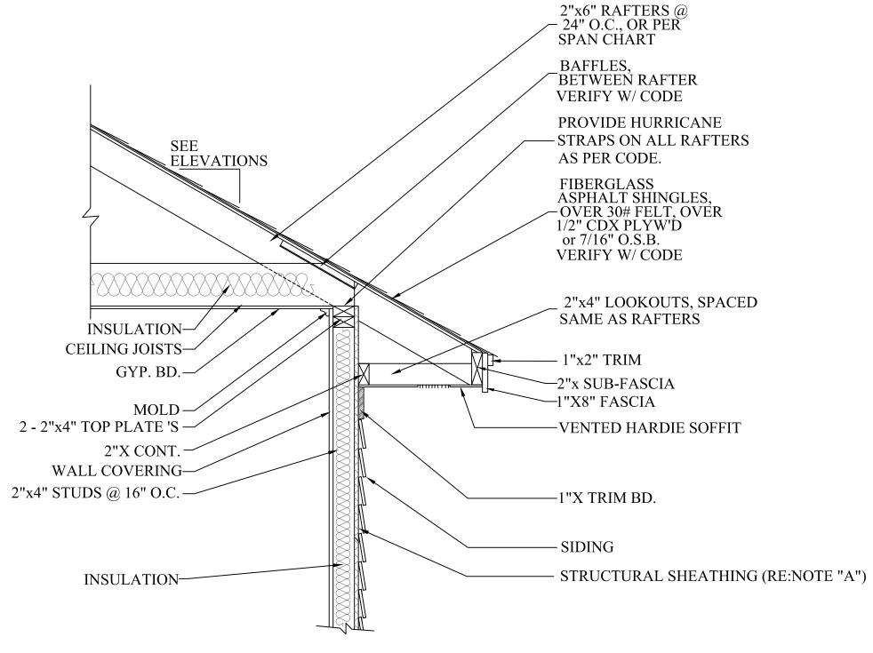
NOTE "A": PROVIDE A MINIMUM OF 7/16" STRUCTURAL WOOD PANEL ATTACHED w/ 8d COMMON OR 10d BOX NAILS AT 4" SPACING ON EDGE AND 12" IN FIELD.
