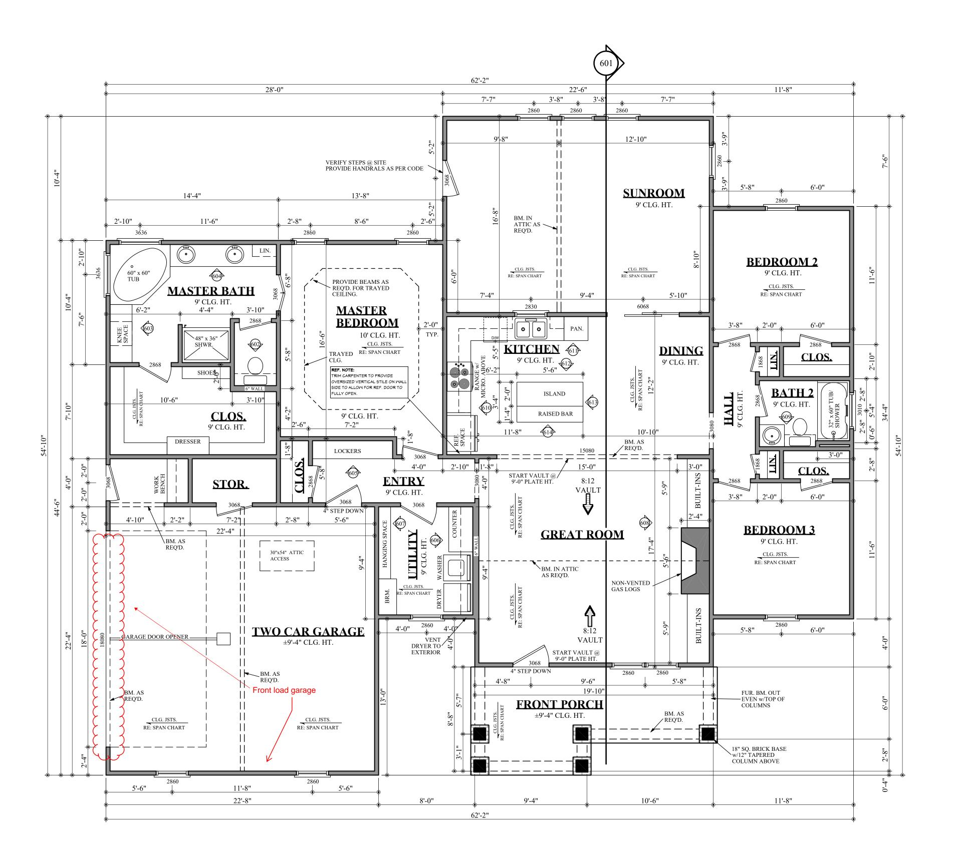
NOTE: CONTRACTOR TO LOCATE WATER HEATER AND HVAC UNITS AT SITE.
