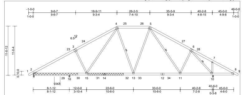
Repair for a crack in the bottom chord where indicated.
