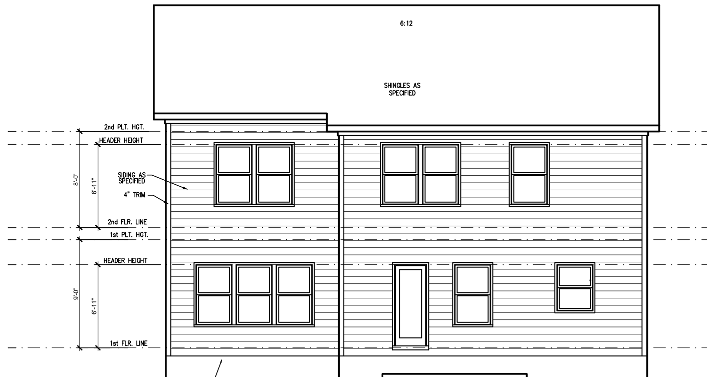
REAR ELEVATION 'TRADITIONAL' (CRAWL)
