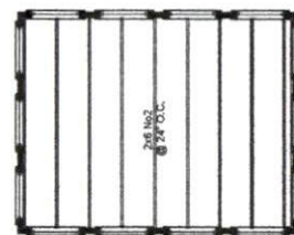
BB 2ND FLOOR CEILING JOIST SCALE: 1/4" = 1'-0"
