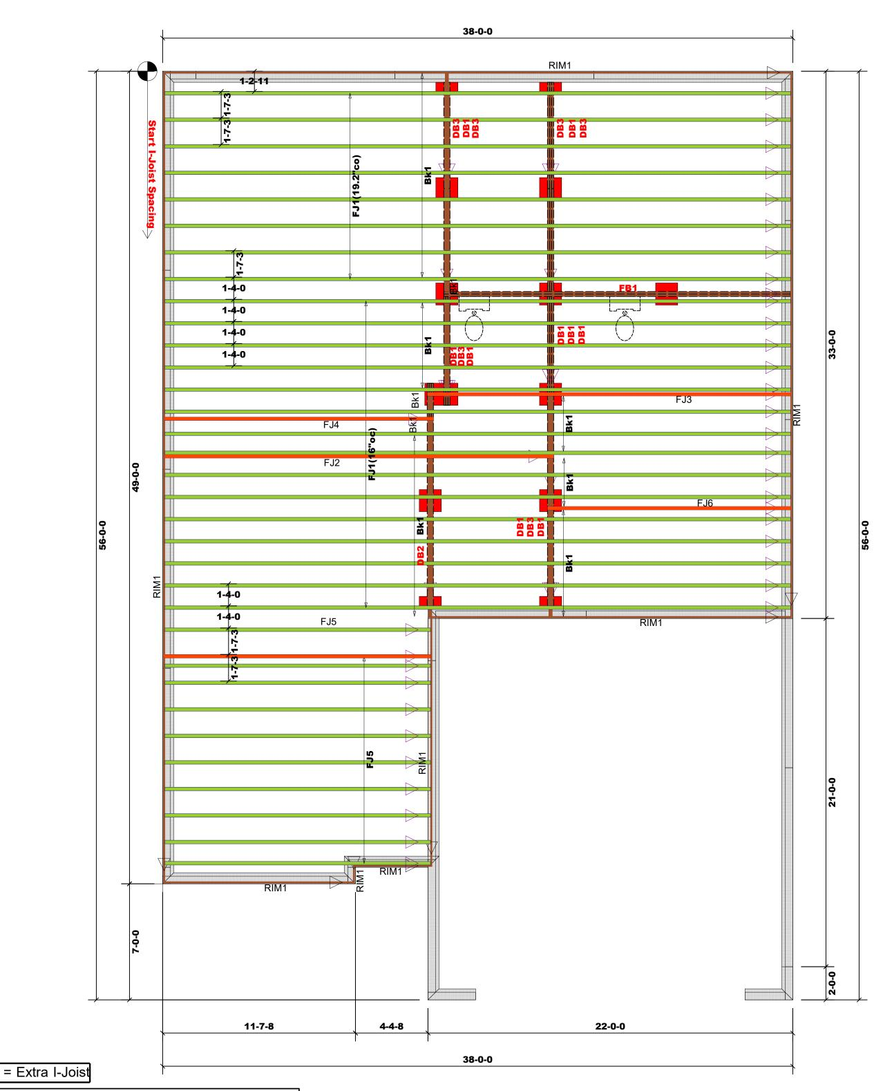
Products Length Plies PlotID Product Net Qty Fab Type FF 37-8-13 11 7/8" NI-40x 23 FJ1 FJ2 23-5-7 FF 11 7/8" NI-40x 1 FF FJ3 11 7/8" NI-40x 21-11-1 FJ4 FF 16-2-7 11 7/8" NI-40x 16-0-6 FF 11 7/8" NI-40x FJ5 11 FJ6 14-8-1 11 7/8" NI-40x FF FB1 21-0-0 1-3/4"x 11-7/8" LVL Kerto-S FF 14-0-0 2x10 SPF No.2 FF DB1 FF 2x10 SPF No.2 DB2 14-0-0 3 DB3 8-0-0 2x10 SPF No.2 FF FF 12-0-0 1 1/8" x 11 7/8" Rim Board RIM1 15 2-0-0 11 7/8" NI-40x
