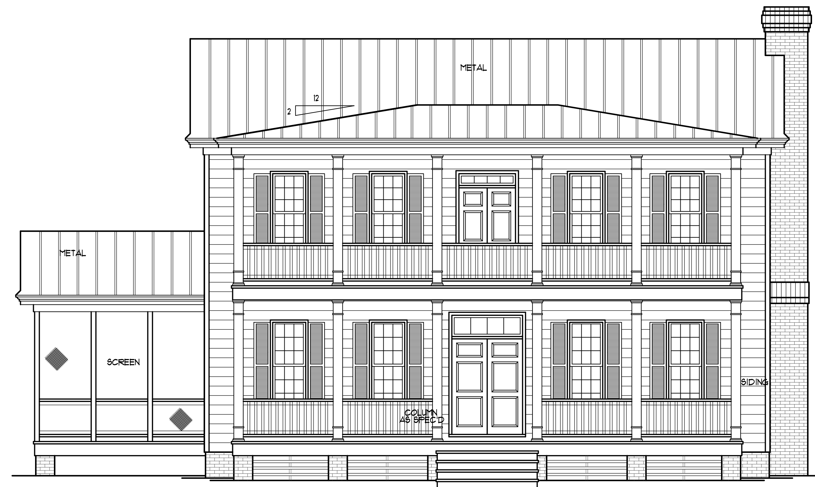
FRONT ELEVATION SCALE: 1/4" = 1'-0"
