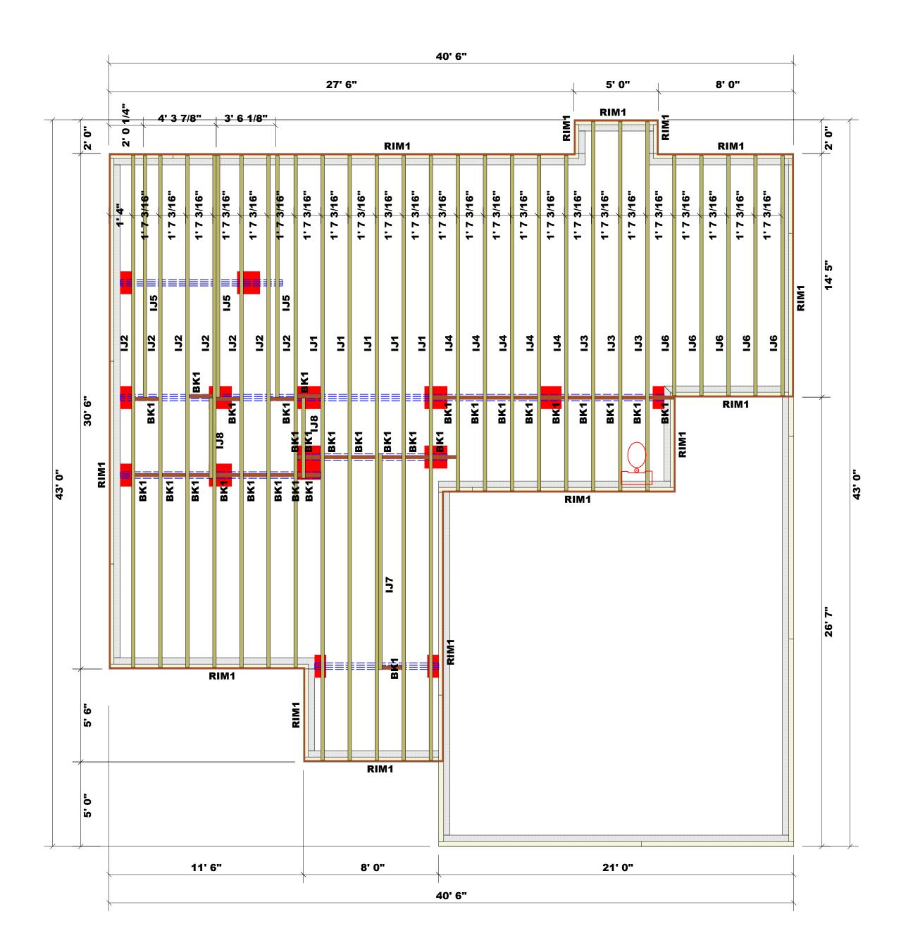
Truss Placement Plan SCALE: 1/4" = 1'
