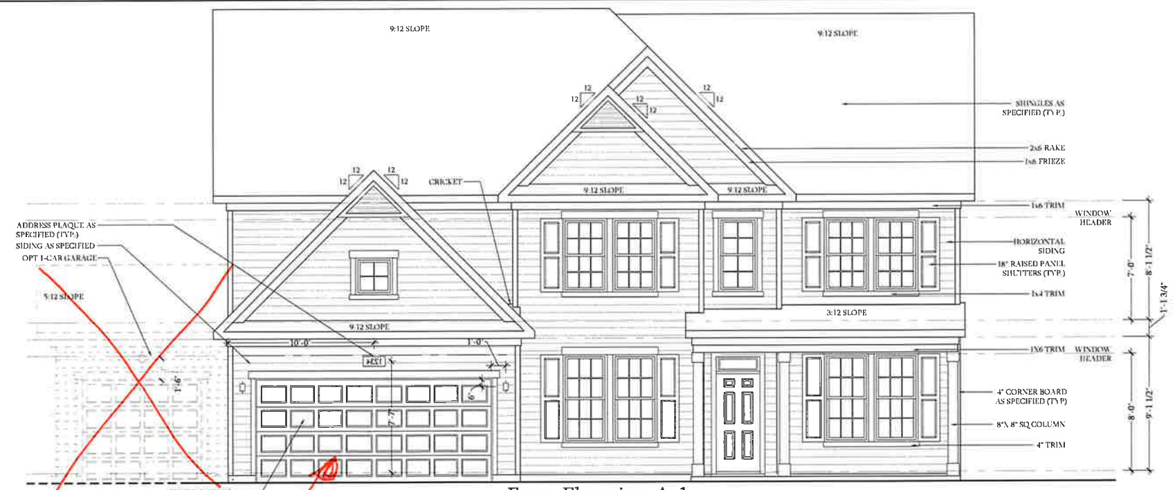
Front Elevation-A-1 SCALE: 1/4"=1'-0" ON 22x34 AND 1/8"=1'-0" ON 11x17
