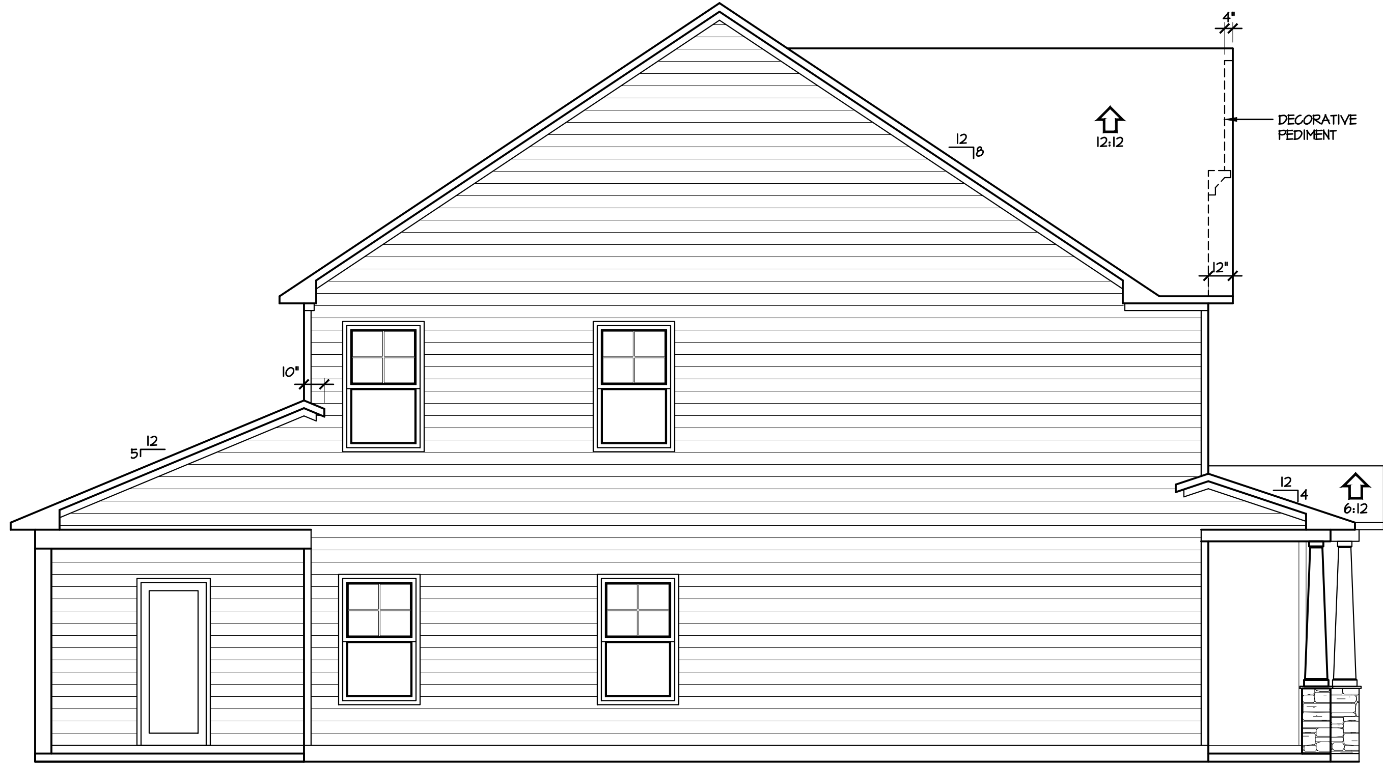
2 LEFT SIDE ELEVATION 1/4" = 1'-0"
