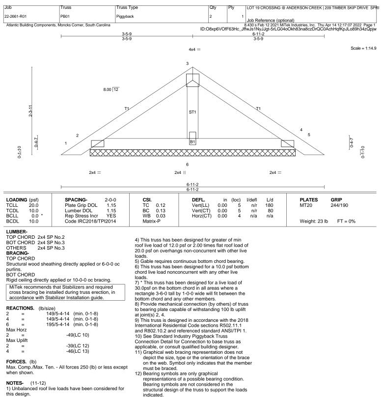
2) Wind: ASCE 7-16; Vult=130mph (3-second gust) Vasd=103mph; TCDL=5.0psf; BCDL=5.0psf; h=23ft; Cat. II; Exp B; Enclosed; MWFRS (envelope) gable end zone and C-C Exterior(2) zone; end vertical left and right exposed;C-C for members and forces & MWFRS for reactions shown; Lumber DOL=1.60 plate grip DOL=1.60
