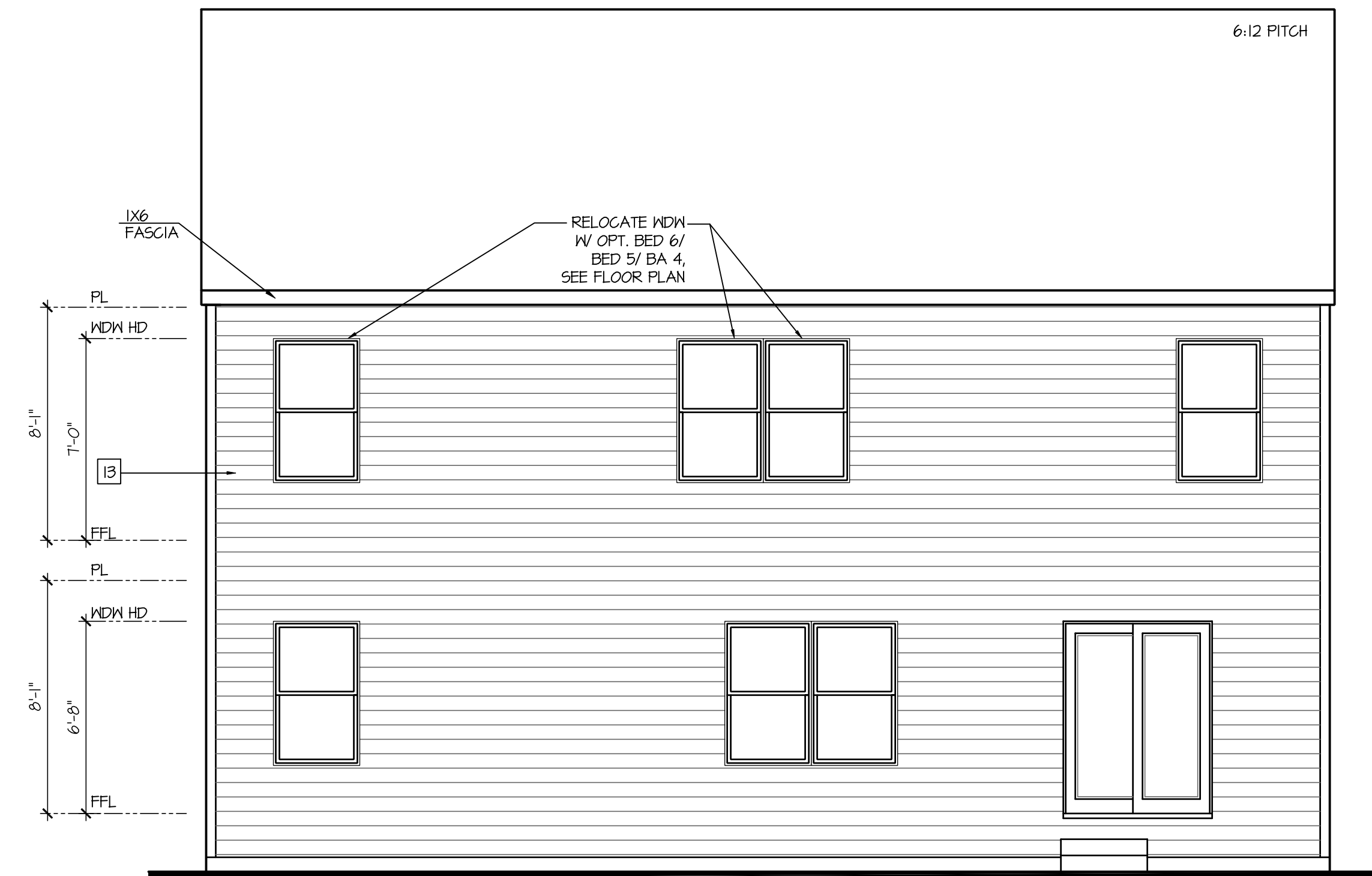
Rear Elevation 'R' w/ Opt Crawl Space SCALE: 1/4"=1'-0" AT 22'X34" LAYOUT 1/8"=1'-0" AT 11'X11" LAYOUT
