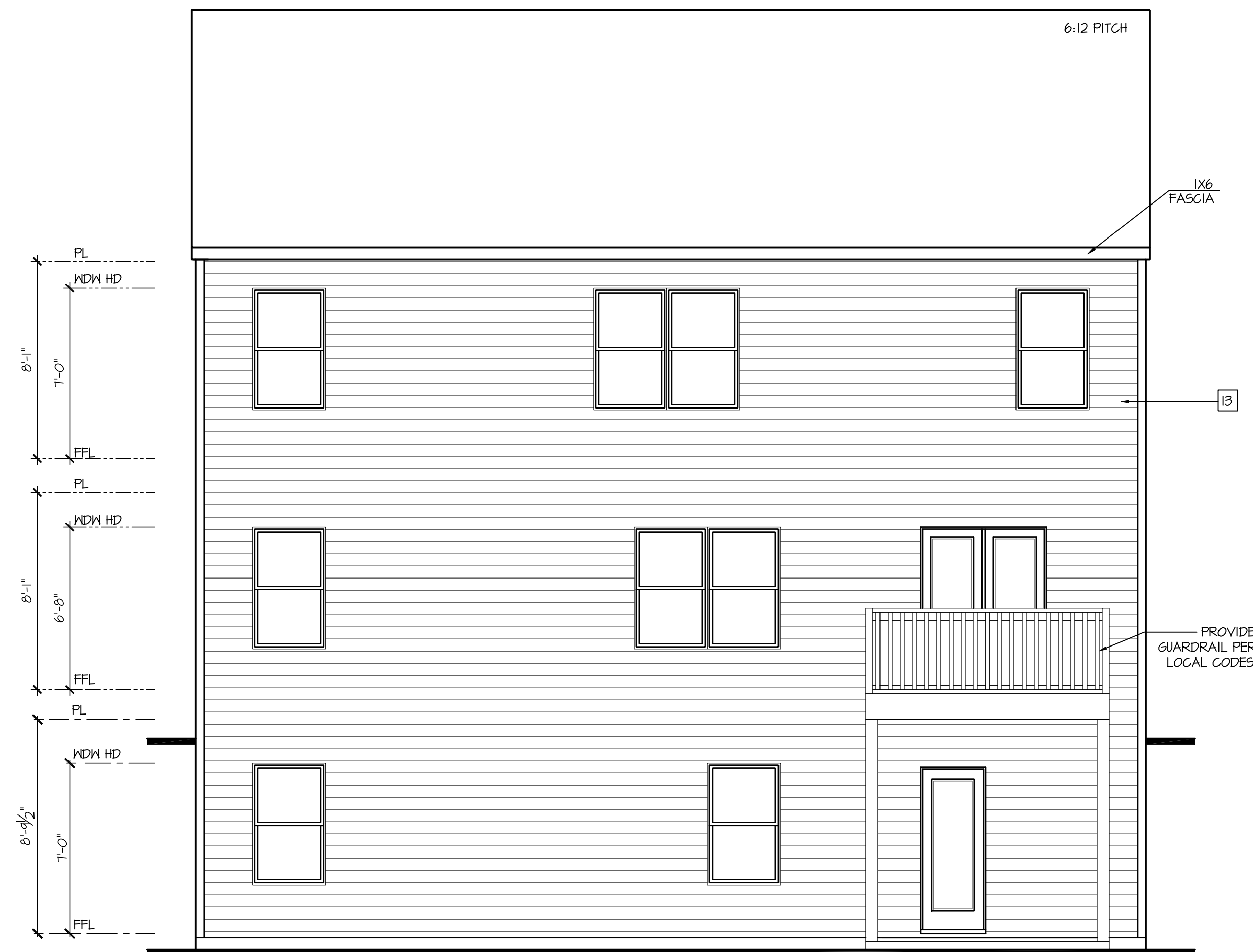
Rear Elevation 'P' w/ Opt Basement SCALE: 1/4"=1'-0" AT 22'X34" LAYOUT 1/8"=1'-0" AT 11'X11" LAYOUT
