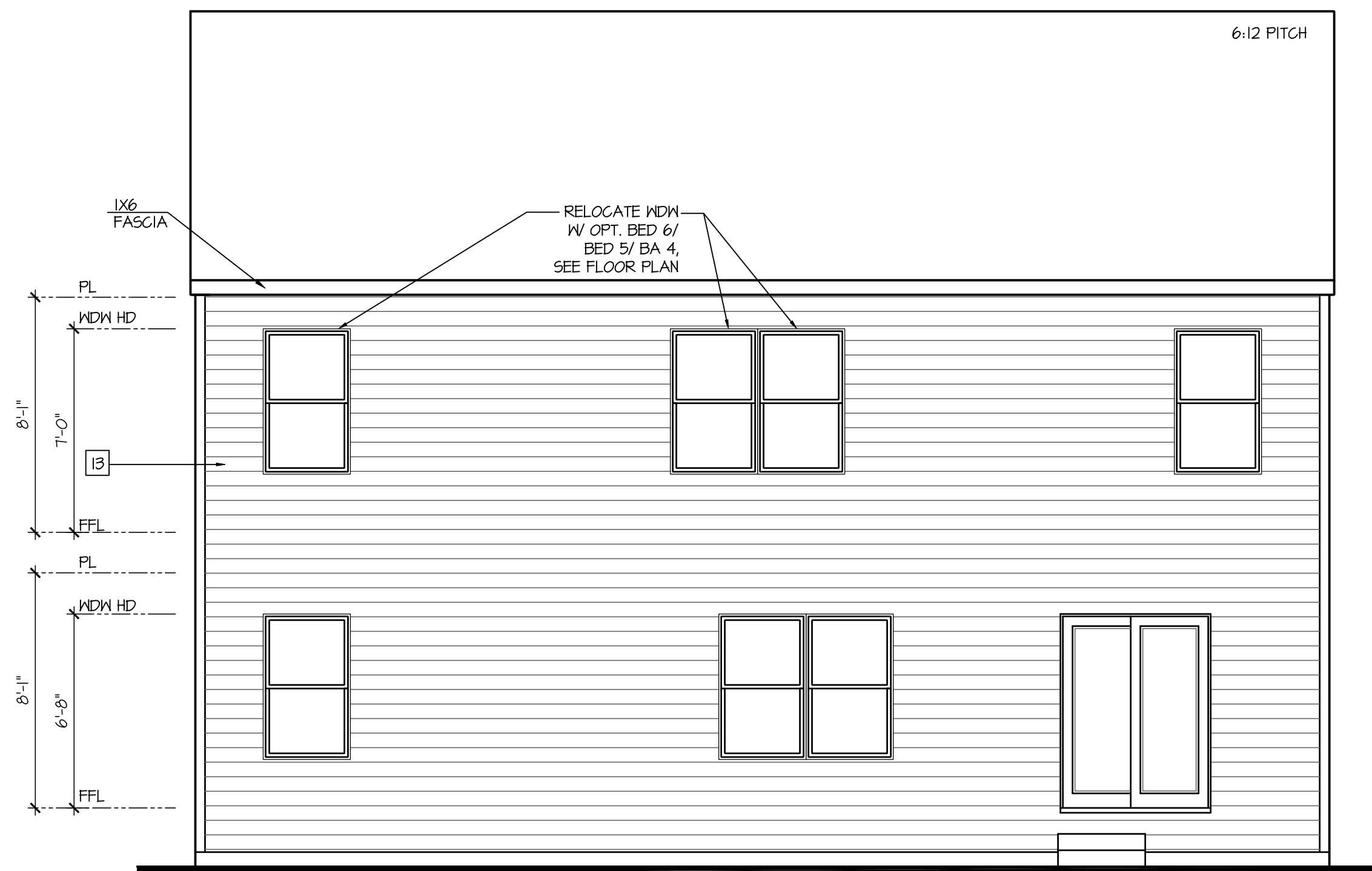
Rear Elevation 'K' w/ Opt Crawl Space
