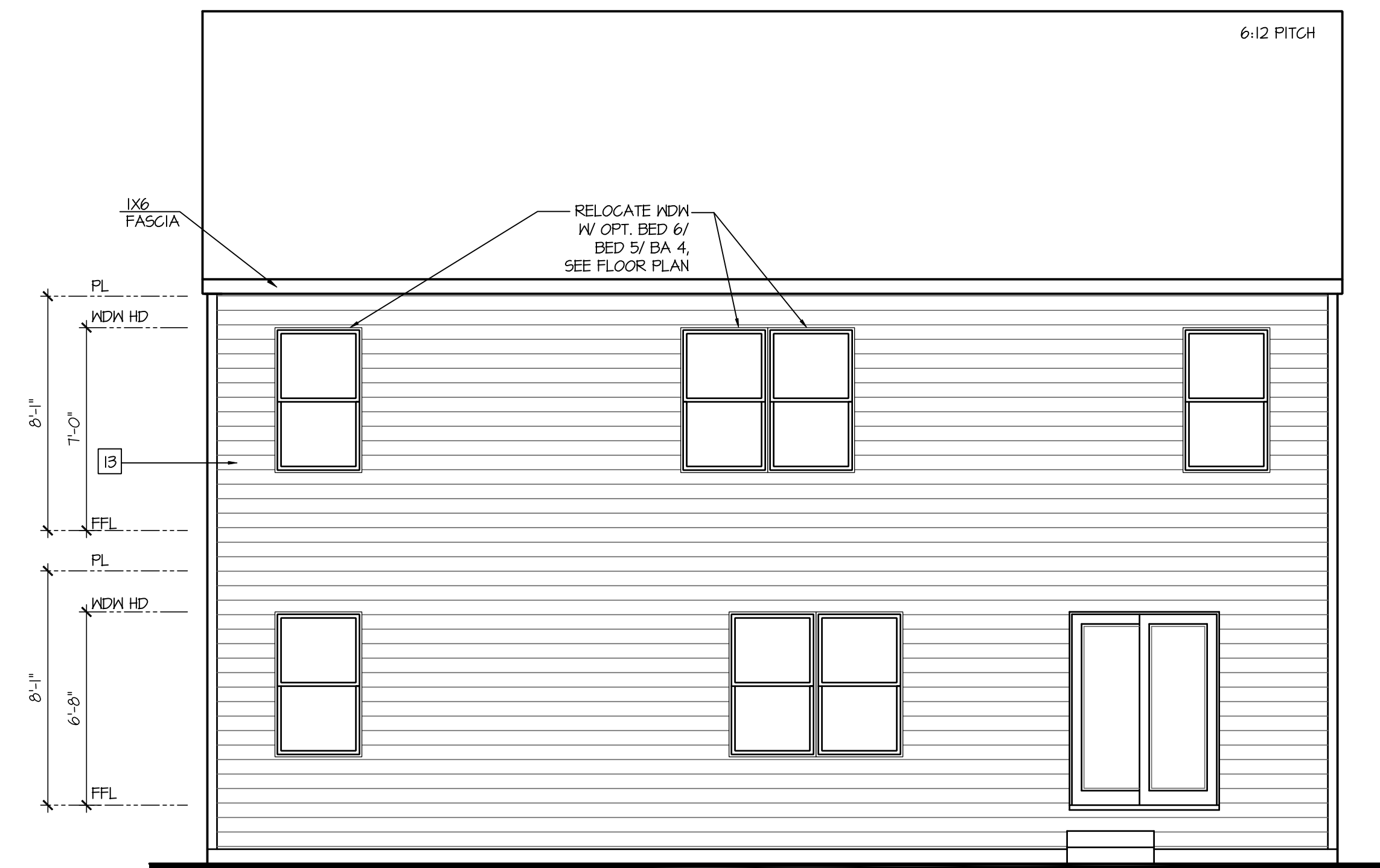
Rear Elevation 'P' w/ Opt Crawl Space SCALE: 1/4"=1'-0" AT 22'X34" LAYOUT 1/8"=1'-0" AT 11'X11" LAYOUT
