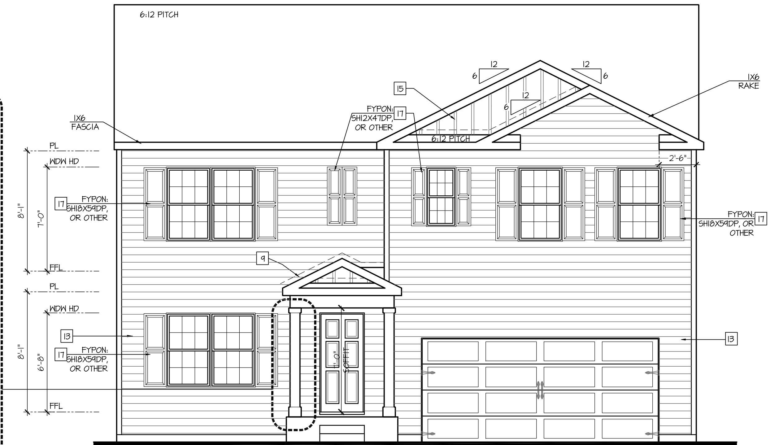
Front Elevation 'A' w/ Opt Crawl Space/ Basement SCALE: 1/4"=1'-0" AT 22'X34" LAYOUT 1/8"=1'-0" AT 11'X17" LAYOUT
