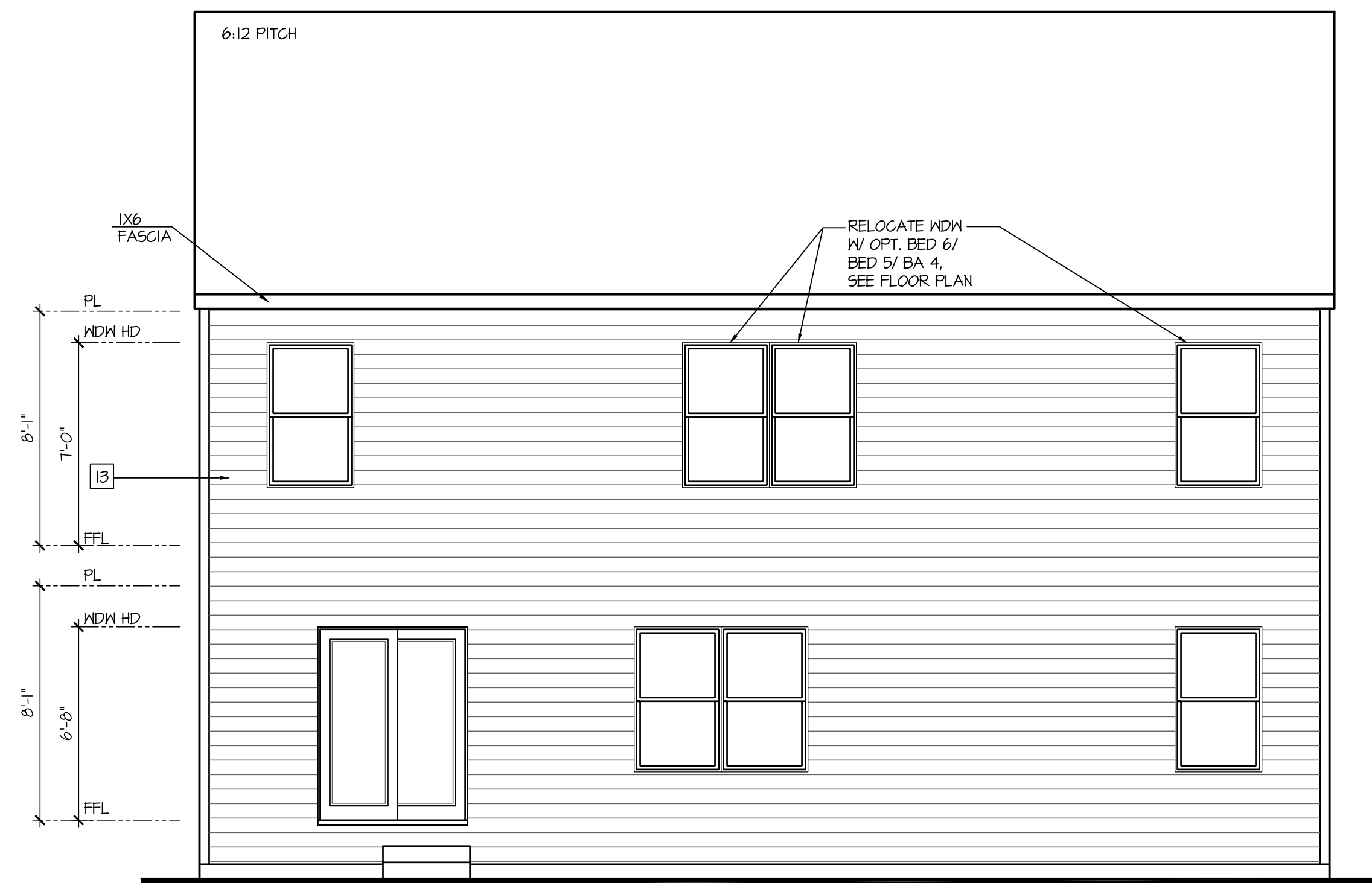
Rear Elevation 'R' w/ Opt Crawl Space
