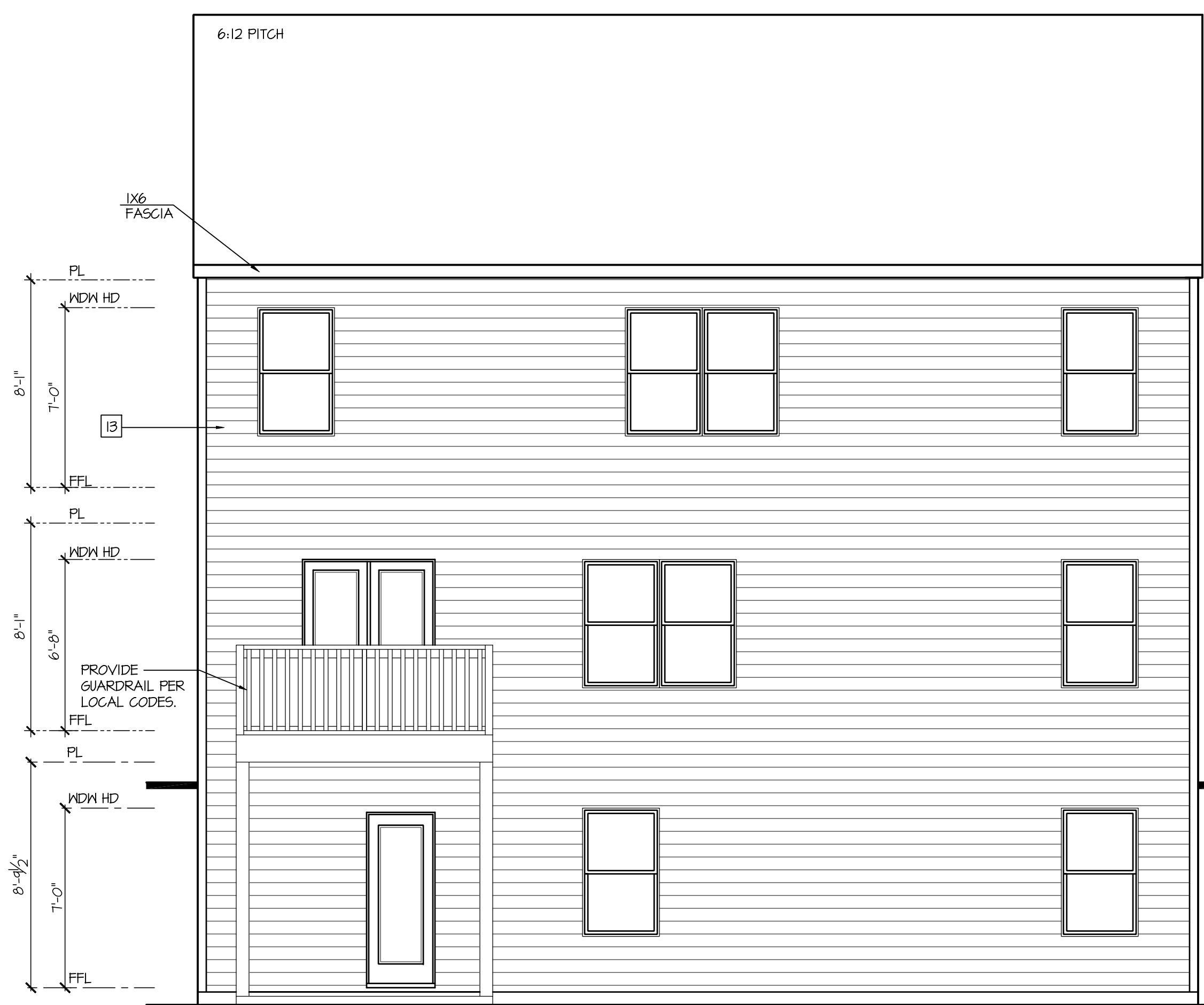
Rear Elevation 'B' w/ Opt Basement SCALE: 1/4"=1'-0" AT 22'X34" LAYOUT 1/8"=1'-0" AT 11'X17" LAYOUT
