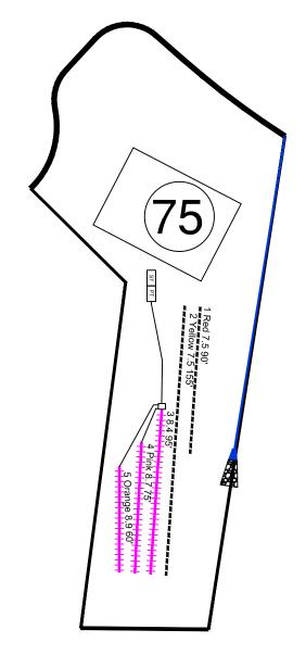
System: Pressure Manifold Lines: 3-5 (230') Accepted Status System 0.4 Soil LTAR 12" Trench Bottom At Grade
