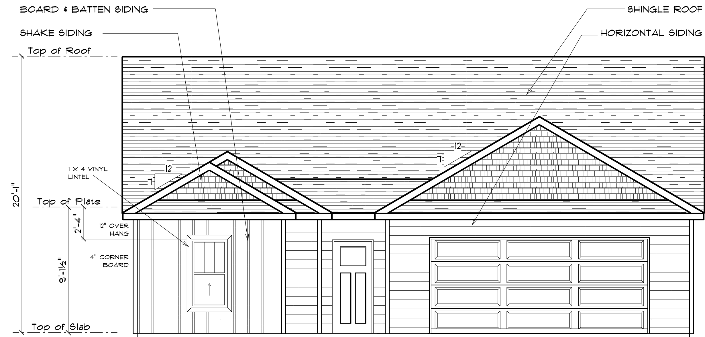
FRONT ELEVATION SCALE: 1" = 1/4"
