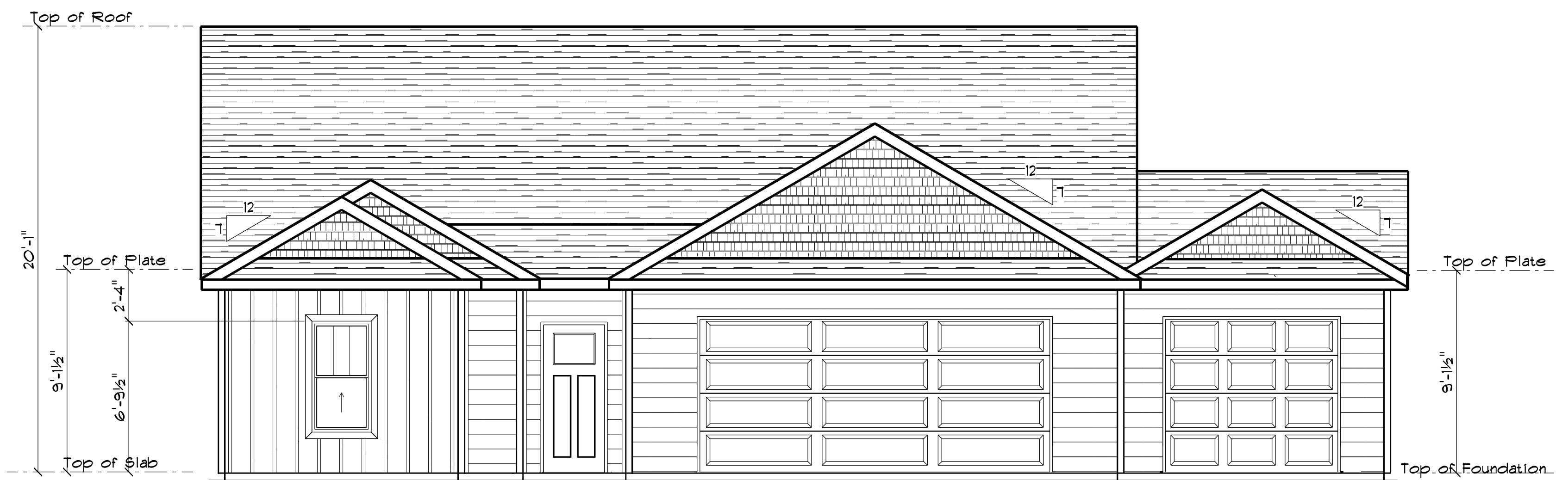
FRONT ELEVATION W/OPTIONAL SINGLE CAR GARAGE SCALE: 1" = 1/4"
