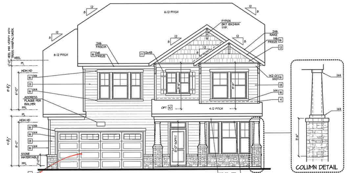
Front Elevation 'B' SCALE: 1/4"=1'-0" AT 22'x34" LAYOUT 1/8"=1'-0" AT 11'x11" LAYOUT Colonial Raised Panel White Garage
